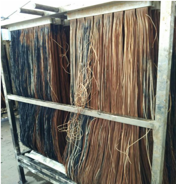
Hollow membrane hardening and wire breakage
